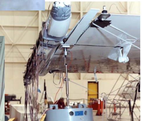
NASA Dryden Flight Research Center Photo Collection http://www.dfrc.nasa.gov/gallery/photo/index.html NASA Photo: EC02-0203-55 Date: August 22, 2002 Photo by: Tom Tschida A thin rod is all that is needed to transmit vibrations from a shaker device (at bottom) and the wingtip of the Active Aeroelastic Wing F/A-18 research aircraft during ground vibration testing
