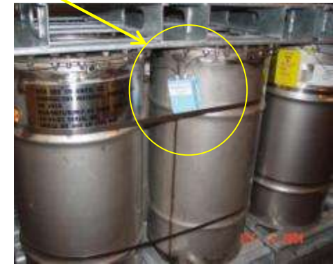
Deployed RF fiber optic seal security sensor on nuclear material containers
