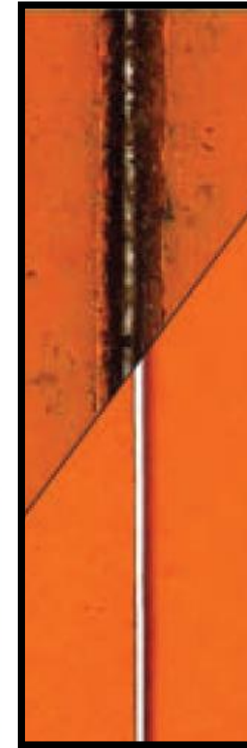
CO 2 (top) vs Nd: YAG (bottom) cut on Kapton
