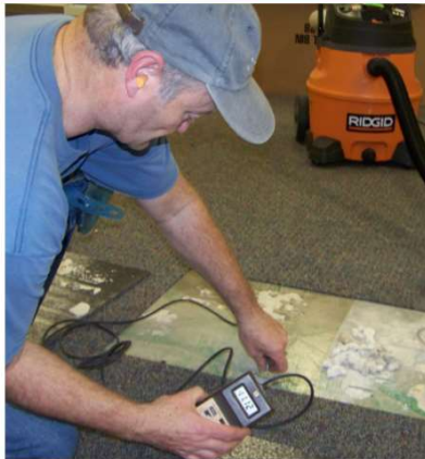
Figure 5. Measuring sub-slab vacuum.
