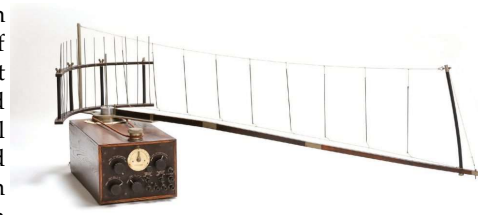
Photograph of Yagi-Uda antenna used as a UHF receiver for a communication experiment from Sendai to Otakamori in 1929 (Citation from web page of RIEC, Tohoku Univ., https://www.riec.tohoku.ac.jp/ja/about-riec/antenna/ ).
