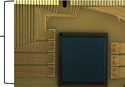
Flip-chip S-MCM attached to PCB for 4K testing
