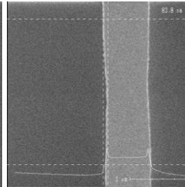
0.8μm line at stitch boundary with 0.25μm overlap
