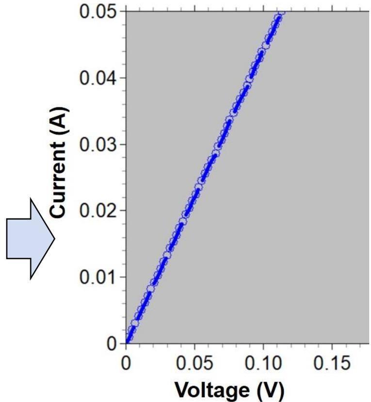
Representative I-V curves of 20x20mm<sup>2</sup> flip-chip daisy chains at 4K
