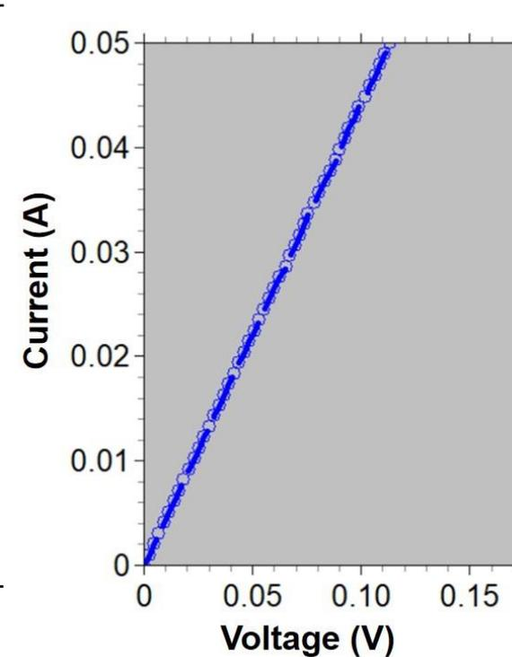
I-V curve of flip-chip S-MCM daisy-chain tested at 4K
