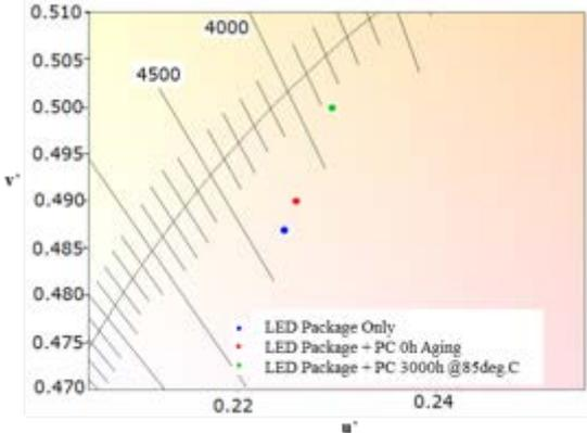
Inconsistent degradation of wavelength-dependent transmittance
