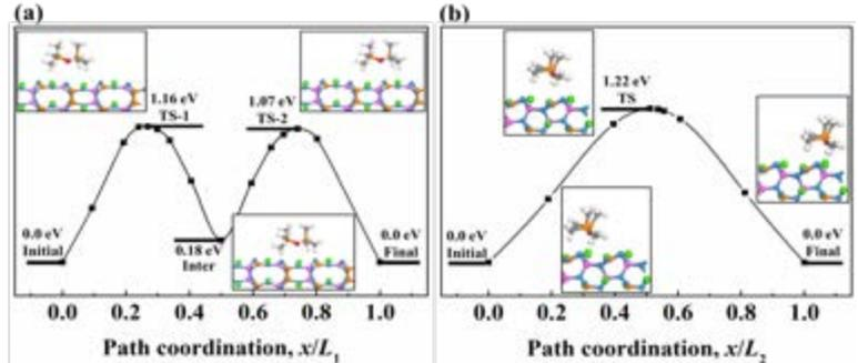
**Pristine CaAlSiN<sub>3</sub>[010] surface**, the minimum-energy pathway along (a) [100] direction. (b) [001] direction.
