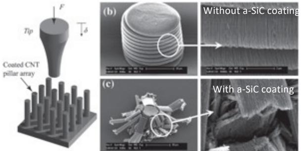
Macroscale phenomena: Different failure modes of CNT pillar with and without a-SiC coating
