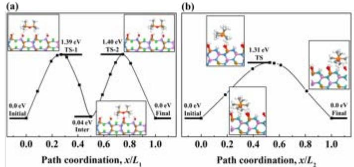
**Hydrolyzed CaAlSiN<sub>3</sub>[010] surface**, the minimum-energy pathway along (a) [100] direction. (b) [001] direction.
