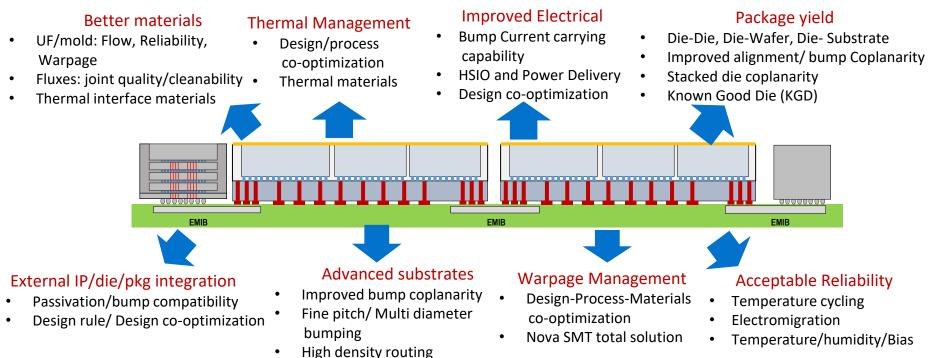
Equipment/ Material/Process/ Design Co-optimization key to Heterogeneous Assembly & Packaging
